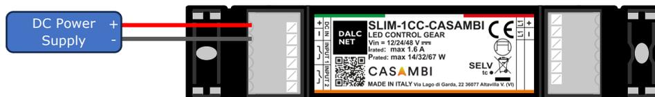
Figure 5: Power Supply Connection Diagram
