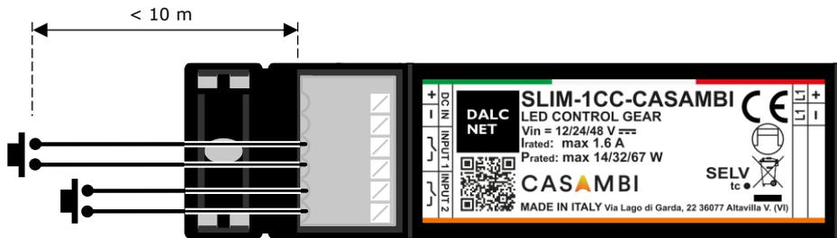
Figure 3: Local Command connection diagram for Short Distances
