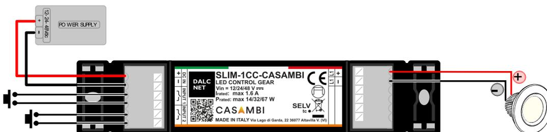
Figure 2: Connection diagram for White or Single-Colour LED loads
