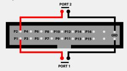
To activate a port, a brief contact of at least 1/25 second must be established between the ports (1...16) and the ground (GND) using the external HE20 connector.
