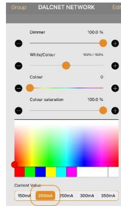
Maximum current that can be supplied by the device for each single output: 200mA
