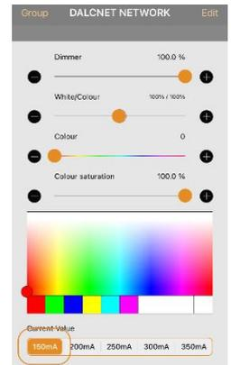
Maximum current that can be supplied by the device for each single output: 150mA
