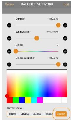
Maximum current that can be supplied by the device for each single output: 350mA
