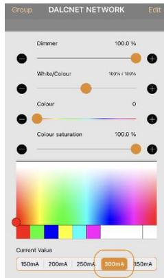
Maximum current that can be supplied by the device for each single output: 300mA
