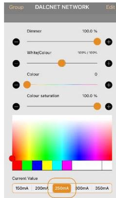
Maximum current that can be supplied by the device for each single output: 250mA
