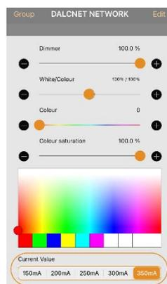
8. Inside of the device configuration, a function bar will appear where it can set the desired current.
