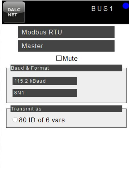
The screenshot shows the configuration page for BUS 1 in Master mode. The interface includes a 'DALC NET' logo and 'BUS 1' with a blue status indicator. The 'Modbus RTU' section is set to 'Master'. There is a 'Mute' checkbox which is currently unchecked. The 'Baud & Format' section shows '115.2 kBaud' and '8N1'. The 'Transmit as' section has a radio button selected for '80 ID of 6 vars'.
