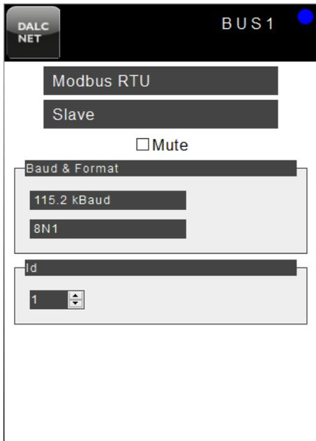
The screenshot shows the configuration page for BUS 1 in Slave mode. The interface includes a 'DALC NET' logo and 'BUS 1' with a blue status indicator. The 'Modbus RTU' section is set to 'Slave'. There is a 'Mute' checkbox which is currently unchecked. The 'Baud & Format' section shows '115.2 kBaud' and '8N1'. The 'Id' section has a dropdown menu set to '1'.
