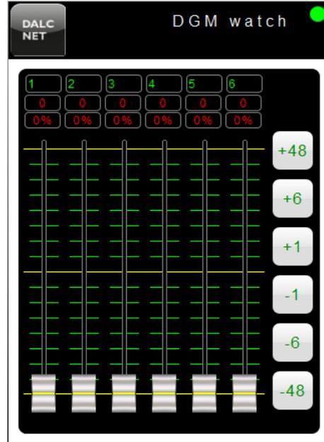
DGM01 provides a WebApp for supervision and setting of all available channels, which can be used from every modern device with an HTML5 capable browser.
