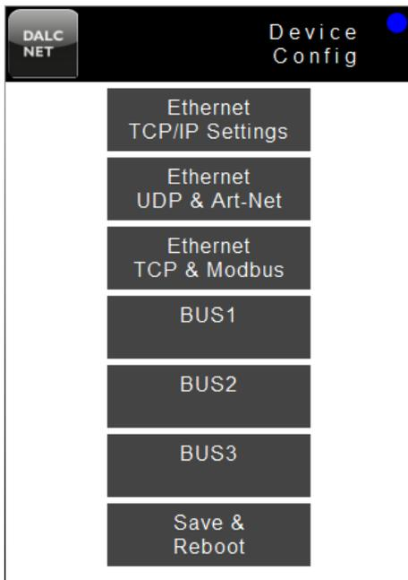
On the main page of the Gateway's Web interface, **Device Config** section is available.
