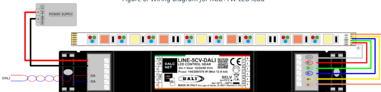
Figure 7: Wiring diagram for RGB+WA LED load
