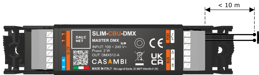
Figure 6: Local Command connection diagram for Short Distances
