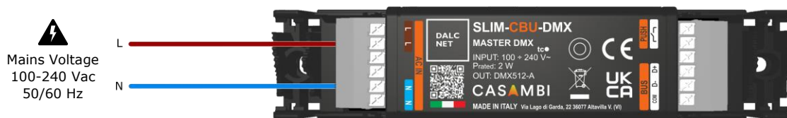
Figure 7: Mains voltage Supply wiring Diagram
