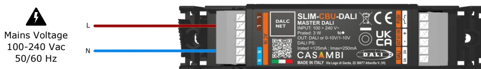
Figure 7: Power Supply wiring Diagram
