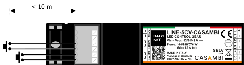
Figure 9: Local Command connection diagram for Short Distances
